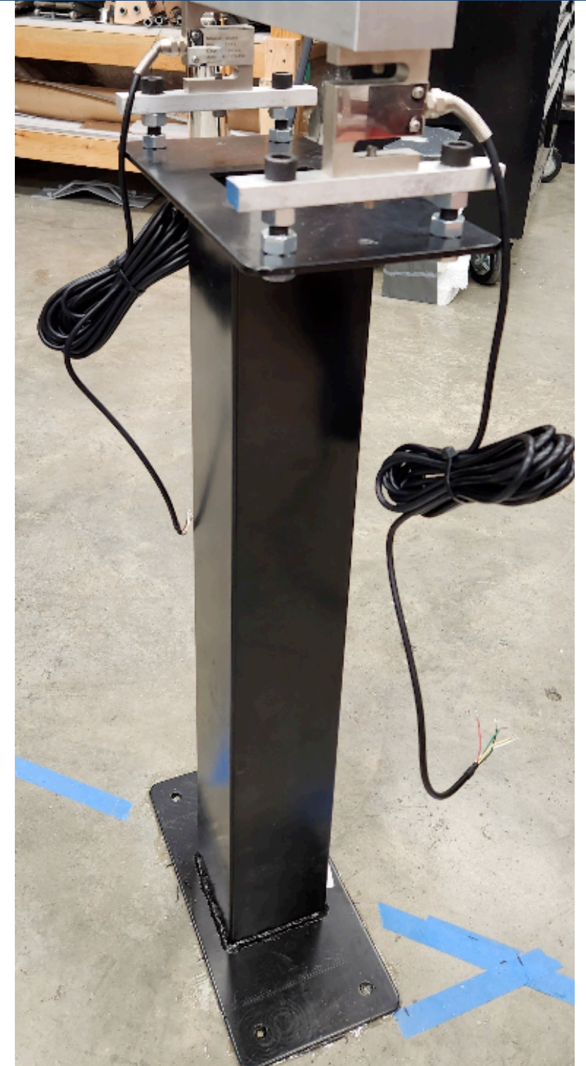
Dual load-cells with support bar on a post for monitoring the weight balance
