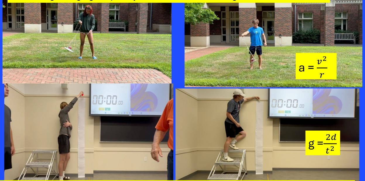
Measuring drop time of pickle ball and ping-pong ball to determine value of g
