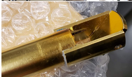
Top: UNH solid-state microwave system; Bottom: Bottom part of waveguide with reflector
