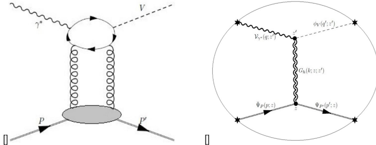
electroproduction of a vector meson probing the **gluon GPD**: (a) leading QCD contribution in the Regge limit; (b) leading Witten diagram in the large- $N_c$  limit.
