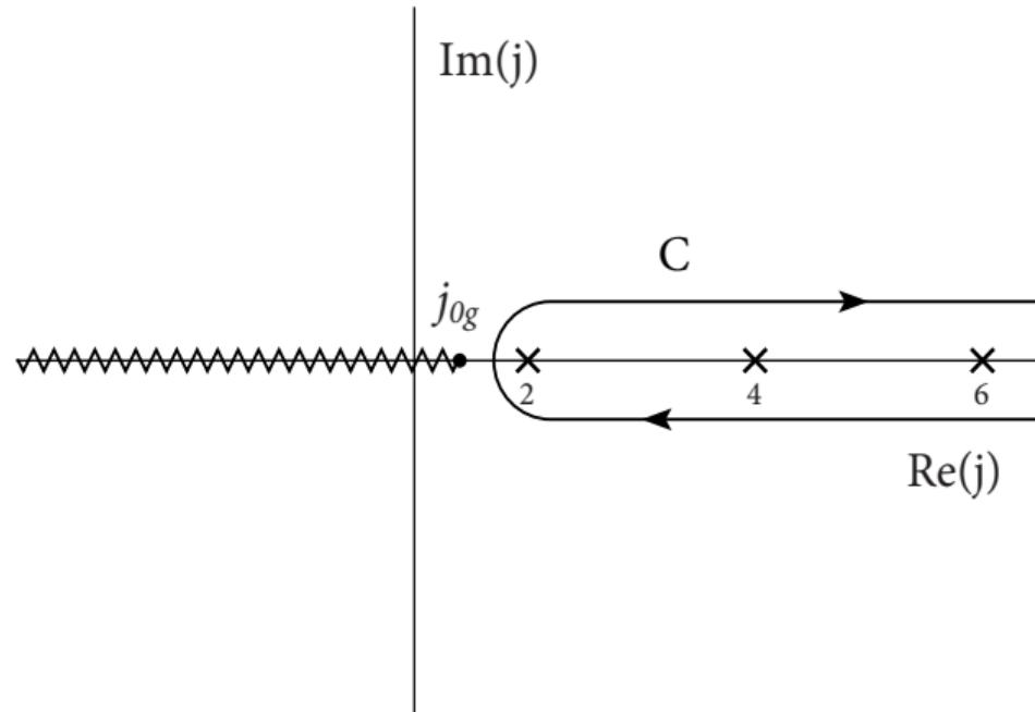
Illustration of the integration contour  $C$  in the complex  $j$ -plane used for computing the contour integral with a branch cut displayed for  $\text{Re}(j) \leq j_{0g} = 2 - 2/\sqrt{\lambda}$ .
