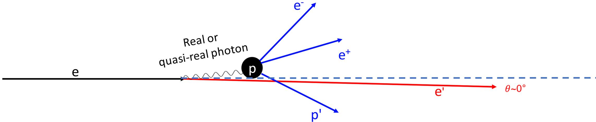
The kinematics of the scattered beam electron is identified as the missing 4 momentum of the e<sup>-</sup>e<sup>+</sup>p' system with  $Q^2 \sim 0$  and  $M_{\text{mis}} \sim 0$
