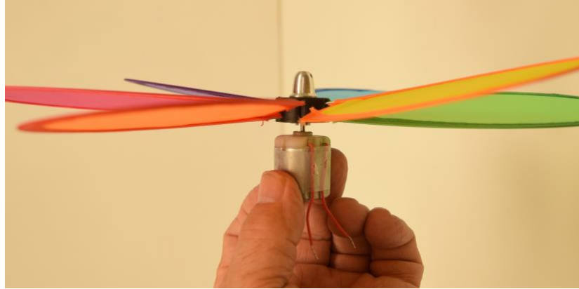
Fig. 10.4.3. Assembled propeller, cowl, and motor
