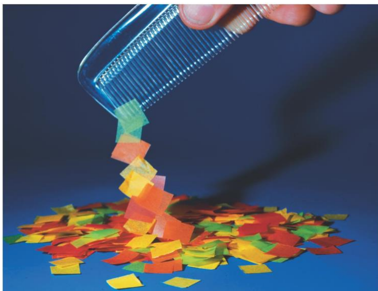
Fig. 3.6 A charged comb causes polarization of charge within neutral pieces of paper
