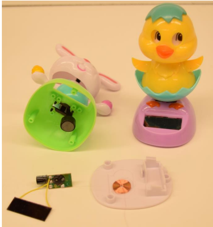
Fig. 10.4.2 View of 4 basic components of the dancing toy.
