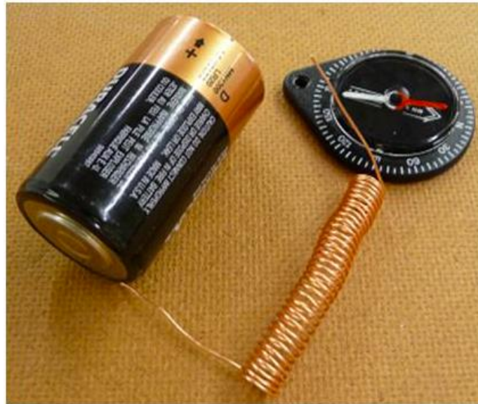
Fig 7.1.1 The wire is fashioned into a solenoid. Note that since the positive terminal of the battery is not connected to the solenoid, there should be no current in the wire.
