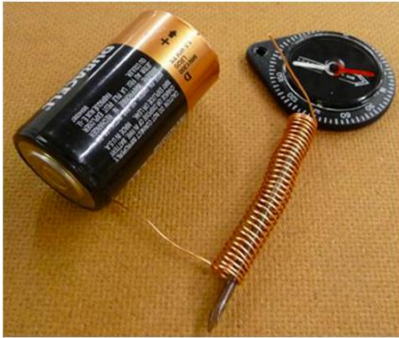
Fig 7.1.2 A nail is now inserted into the solenoid.
