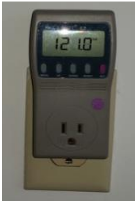
Fig. 2.3.1 The power meter plugs directly into a standard electrical outlet.
