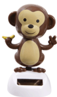
Fig. 10.4.1 Examples of solar powered dancing toys. In each case there is a solar photovoltaic cell attached to each toy (black looking rectangle).
