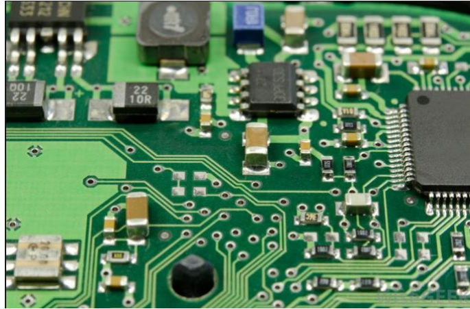
Fig. 9.0.1 The light colored lines are conductive and serve as the wires on this circuit board. (Image from wisegeek.org)
