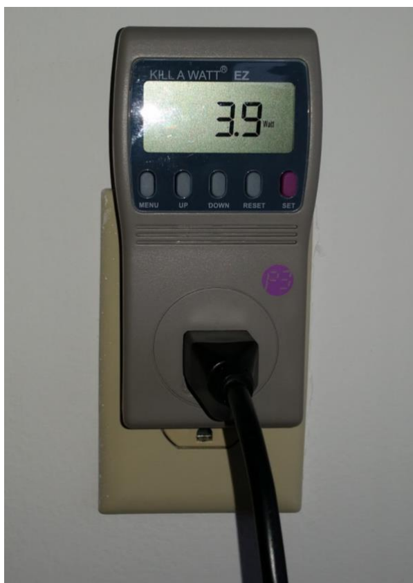
Fig. 2.3.2 The device plugged into the meter is converting electrical energy into other types at a rate of 3.9 Joules per second, or Watts.
