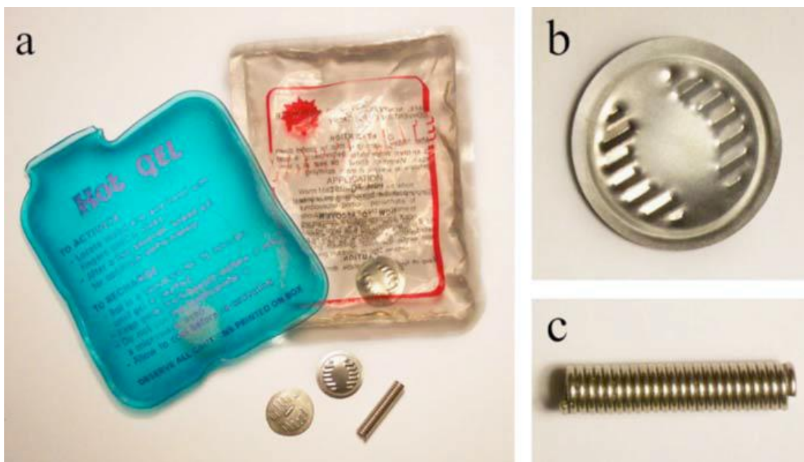
Fig. 1.2.1a. The “hot gel” and “warm mate” heat pads and a selection of triggers. Close up images of b the flexible disc and c the spring type trigger. The flexible disk trigger is 19 mm in diameter and is the type in your gel pad.
