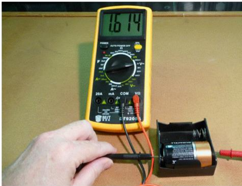
Fig. 8.1.2 The multimeter is measuring the voltage of a single D battery.
