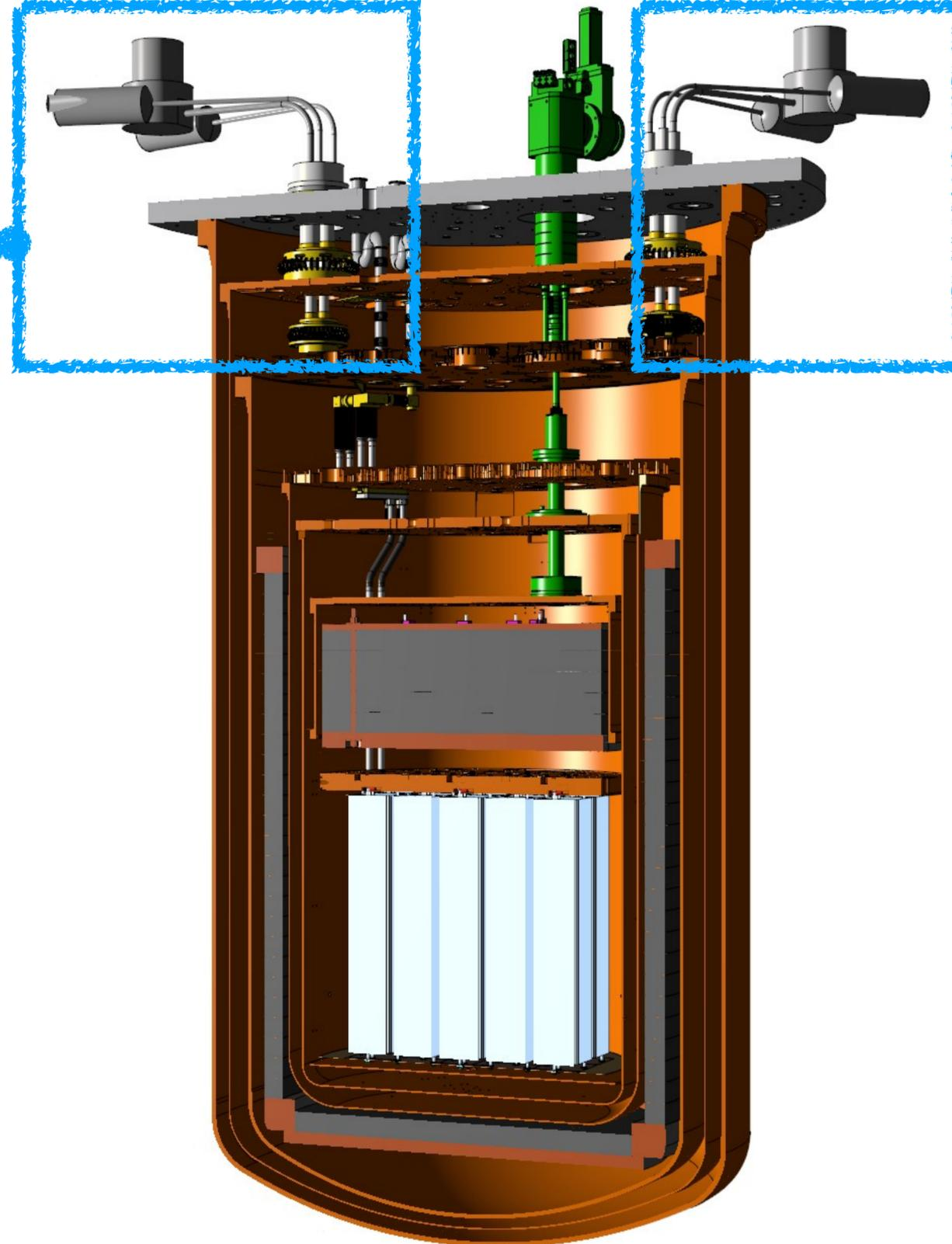
5x pulse tube cryocoolers
