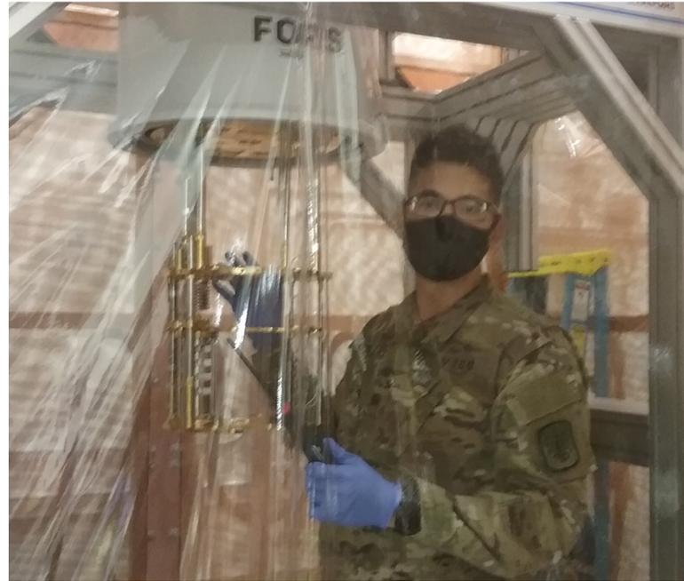
Undergraduate A. Brown installing noise thermometer
