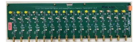
Front End Board for SiPM-based Ecal
