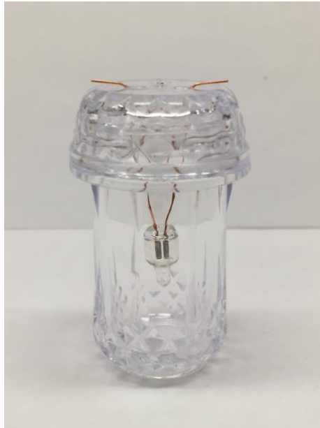
Fig. 7 A mini salt/pepper cannister with a neon gas filled bulb with wires from its anode and cathodes protruding from the holes in the top
