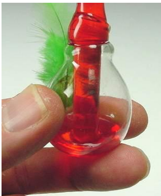
Fig. 2 Instructor using fingers to warm the fluid inside the bulb
