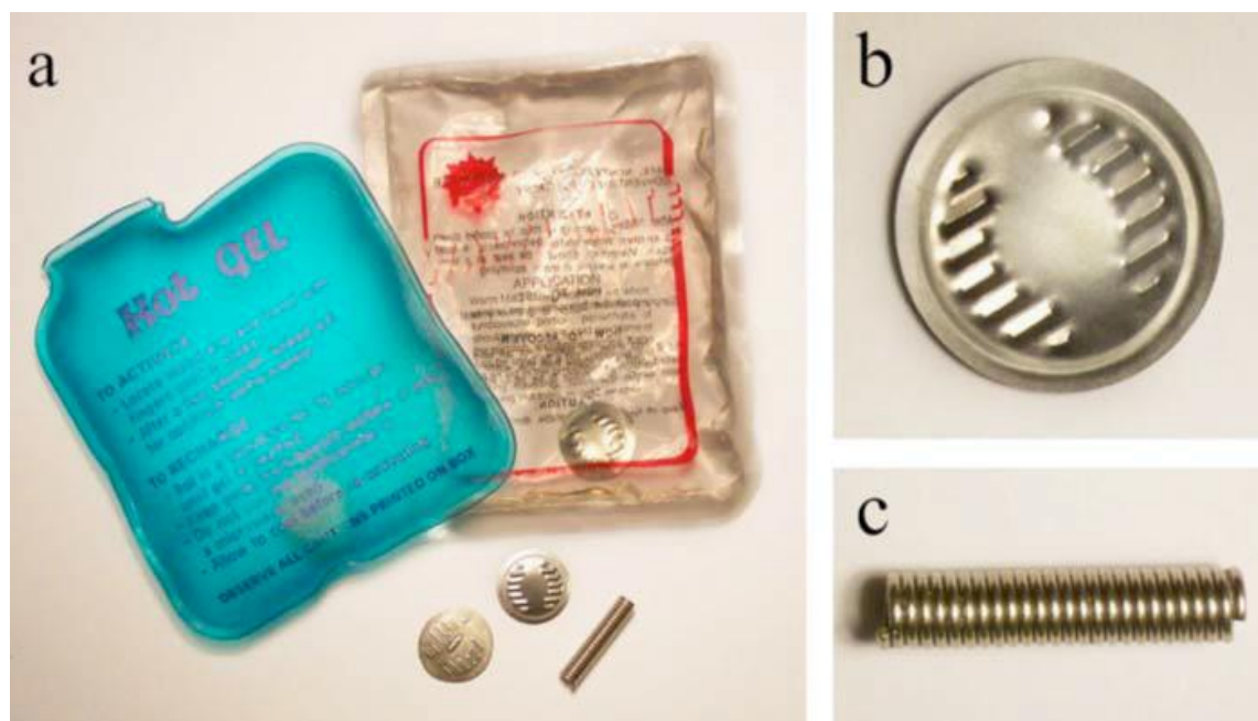
Fig 1a,1b, and 1c Hot gel and warm mate pads, flexible disk trigger, and spring-type trigger.
