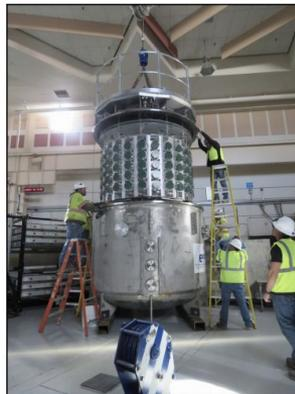
PMTs mounted in PDS boxes at Fermilab
