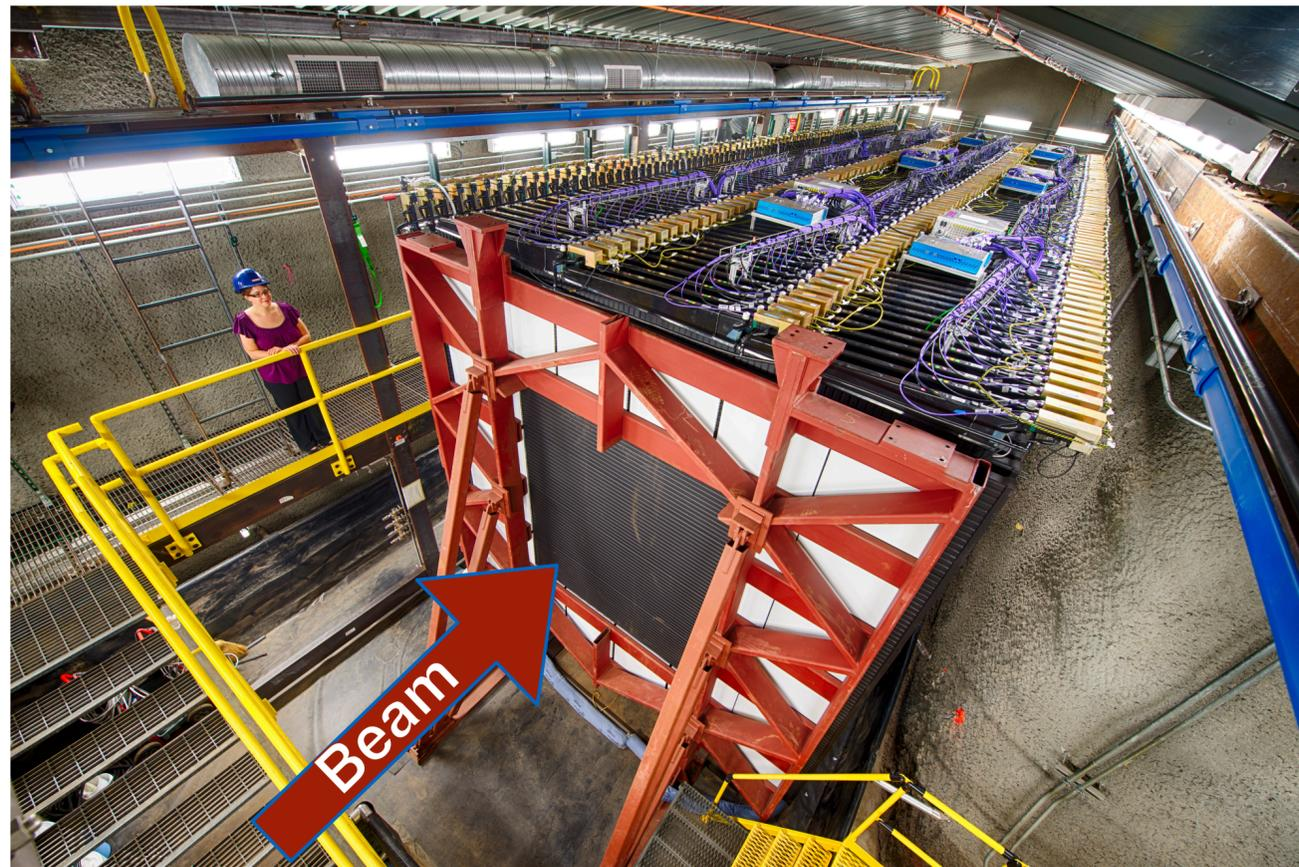
PVC cells filled with **liquid scintillator**, **193 ton** fully active mass and 97 ton downstream muon catcher
