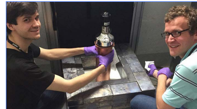
16 kg NaI detector from COHERENT collaboration
