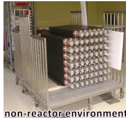
Fig. 3 : Full ISMRAN being integrated for cosmogenic background measurement in a non-reactor environment.
