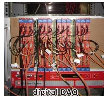
Fig. 4 : Digital DAQ system using 16 ch, 500 MS/s, CAEN digitizers. Pulse processing, triggering and coincidences build on FPGA on board.
