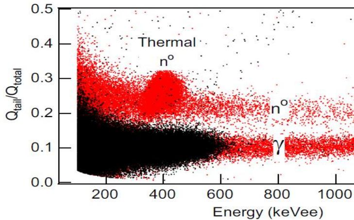
EJen LLNL based EJ-200  ${}^6\text{Li}$  PSD characterization as measured at Virginia Tech
