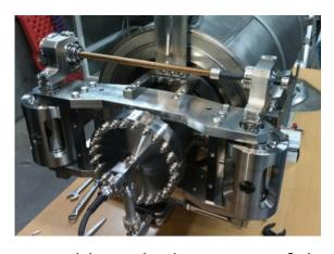
Assembly and adjustment of the Main power couplers conditioned cold tuning systems
