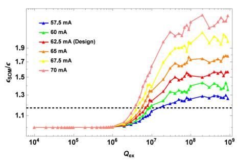
The total emittance growth in ESS linac observed due to longitudinal SOMs. Qs of ESS cavities ~10<sup>5</sup>
