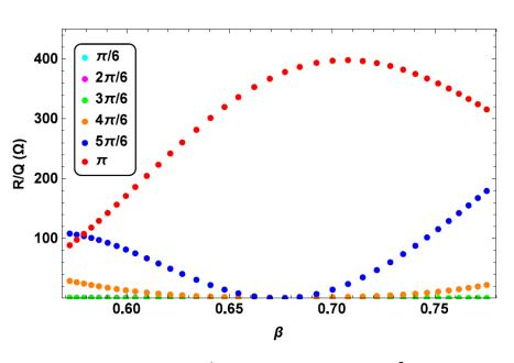
Medium  $\beta$  section, R/Q (proportional to  $V_{acc}^2$ ), for different SOMs
