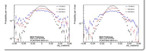
$\bullet$  Measurement of scattering at each nominal momentum point following the deconvolution procedure - final value is a Gaussian fit to the central -40 to  $+40~\rm mrad$
