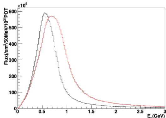
Neutrino energy spectrum for WAGASCI (red, off-axis 1.5 degree), ND280 (black, off-axis 2.5 degree). Peak energy at 1.5 degrees, 800 MeV, vs 600 MeV at 2.5 degrees
