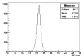
Figure 18: Typical light yield of scintillators in the Proton Module.
