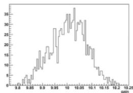
Figure 19: Calibrated gains of MPPCs in the Proton Module.
