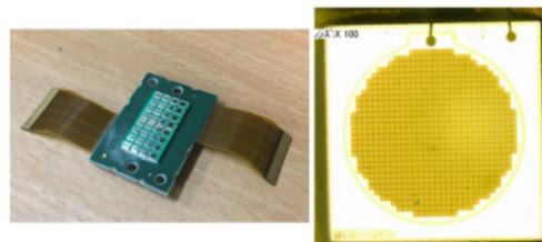
Figure 10: 32-channel arrayed MPPC (left) and an enlarged view of one MPPC channel (right).
