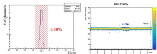
Figure 11: Typical gain distribution (left) and gain history from October 2017 to December 2017 (gains are set to 40 ADC counts) in the WAGASCI module.
