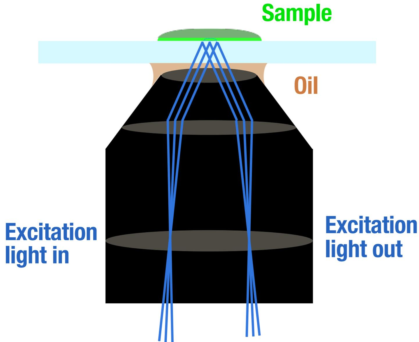
Total internal reflection microscopy (TIRF) is used to image the surface of the sample.
