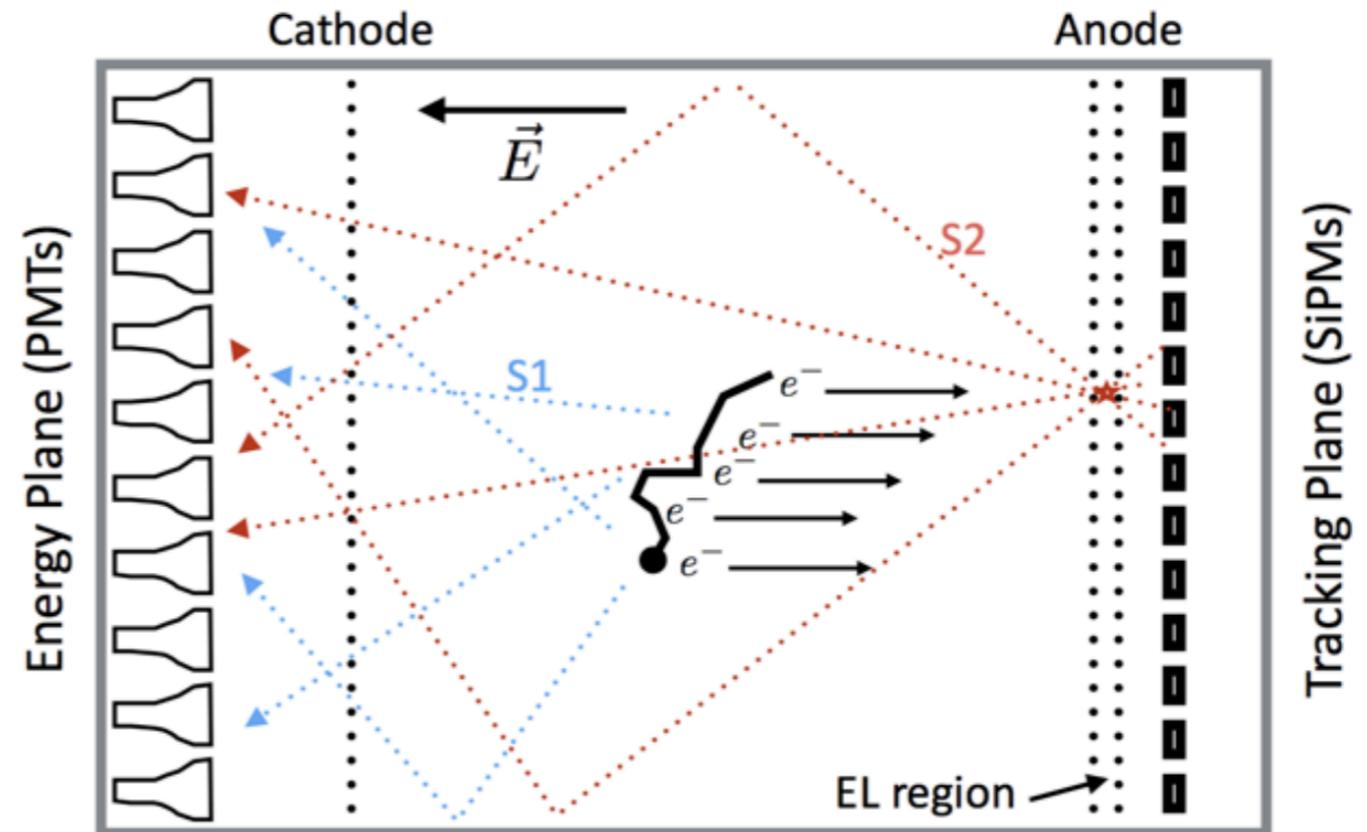
High pressure  $^{136}\text{Xe}$  gas Electro-luminescence TPC
