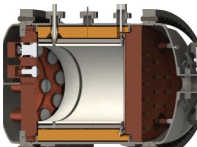
High pressure  $^{136}\text{Xe}$  gas Electro-luminescence TPC
