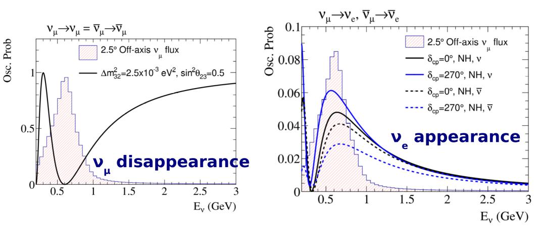
Use of the off-axis technique places a sharp flux peak around the first oscillation maximum
