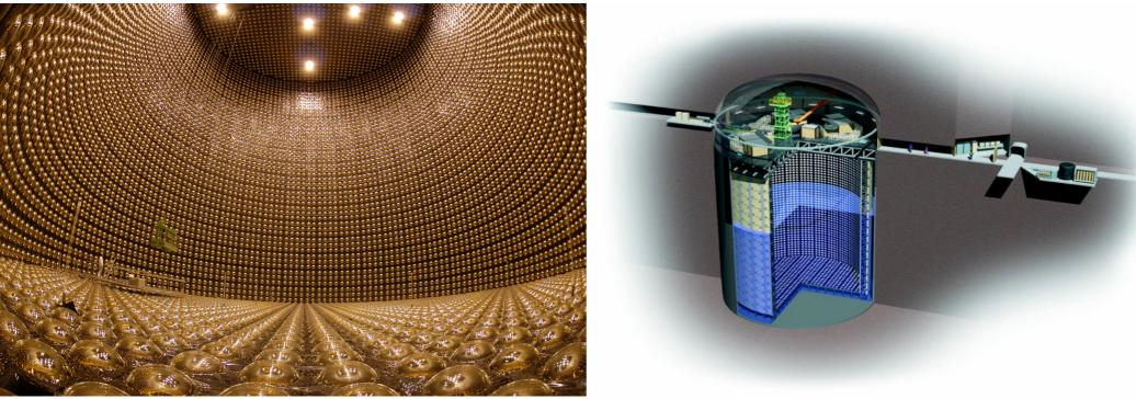
50 kt ultrapure water Cherenkov detector instrumented with 11,000 PMTS in the inner detector for 40% photo-coverage. 1 km underground to reduce background.
