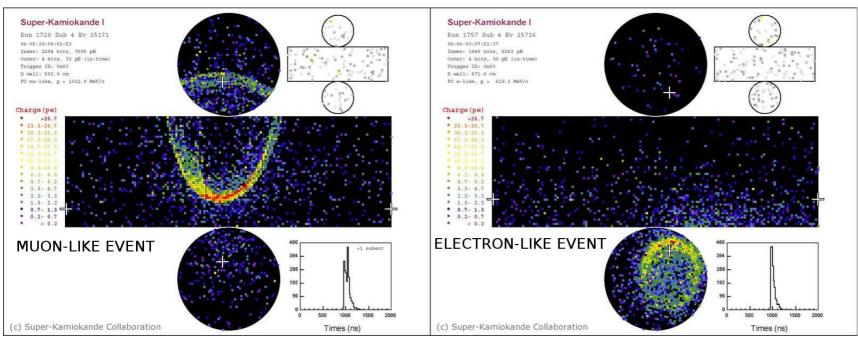
Ring "fuzziness" from scattering: excellent electron-muon separation
