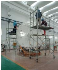
Small prototype of acrylic sphere manufacturing
