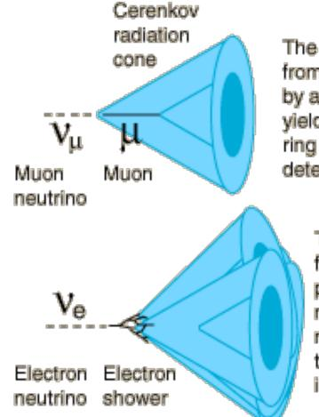
The Cerenkov radiation from a muon produced by a muon neutrino event yields a well defined circular ring in the photomultiplier detector bank.
