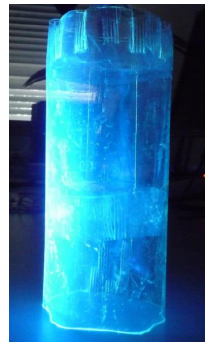
Nylon mini-shroud with wavelength shifter
