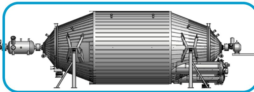
Spectrometer and detector section
