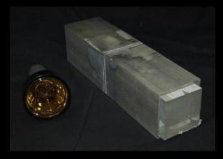
Used <sup>6</sup>LiF:ZnS(Ag) sheets mated to a **solid bar of wavelength-shifting plastic scintillator**. This prototype demonstrated the feasibility of pairing the sheets to wavelength shifting plastic, but the long bars do not have the spatial resolution required for good background rejection
