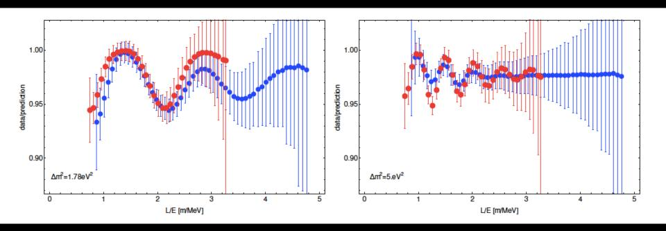
Distribution of events as a function of L/E for two different values of  $\Delta m^2$ . The red data points are for CHANDLER and the blue data points are for SoLid. Resolutions are fully included and the error bars represent the statistical errors after background subtraction.
