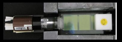
The <sup>22</sup>Na Compton edge is at 1.06 MeV, and at two cubes from the PMT it reconstructs at channel 20, which corresponds to an energy resolution of 6.5%.
