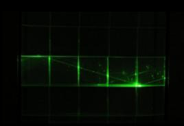
The Raghavan Optical Lattice (ROL), invented by the late Virginia Tech professor, Raju Ragahvan, divides a totally active volume into cubical cells that are read-out by total internal reflection. LENS was designed for solar neutrino detection and not optimized for reactor antineutrino detection.
