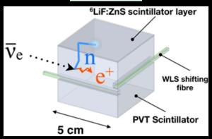
Optically isolated cubes, mated to <sup>6</sup>LiF:ZnS(Ag) sheets, are used to tag IBD. Light is read-out by wavelength shifting fibers in orthogonal directions. It has the spatial resolution of the ROL optimized for reactor antineutrino detection. The small cross-sectional area of the fibers limits the light collection, dilutes the energy resolution and lowers the efficiency.
