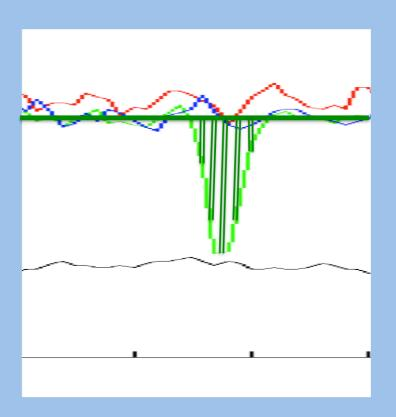
When a hit occurred the peak was immediately located. The are between this curve and pedestal were approximated by integrating. This integration represented the hit's ADC count/value, analogous to the energy deposited within the scintillator
