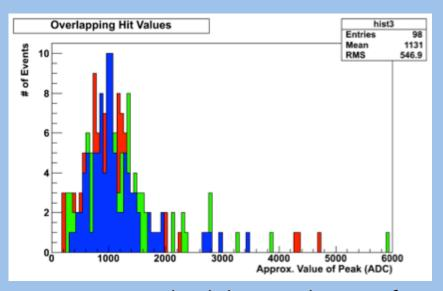
For coincidental hits, it cannot be the same gamma ionizing, so it must be correlated hits by separate yet similar particles. It could be random coincidence, but it is unlikely. It could also be a result of thermal neutrons/gammas from the generator or from background. From this analysis, it is uncertain.
