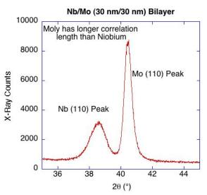
Based on work by Claassen et al., RSI 62, 996(1991)
